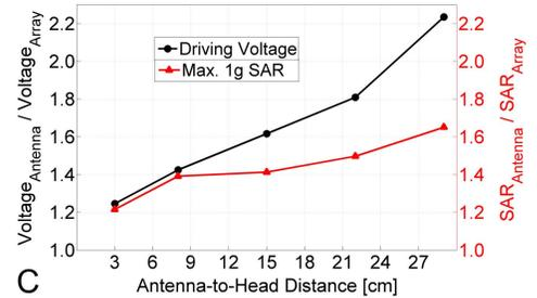
**Figure 1:** Antenna (A) and the tuning/matching circuit (B) of one channel. Fig. 1C shows the driving voltage (black) necessary to scale the  $B_1^+$  field to a reference value when the antenna is placed at various distances to the head as well as the resulting SAR (red).
