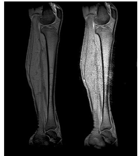
Figure 2. Entire leg images acquired with whole-body coil (left) and waveguide approach (right).
