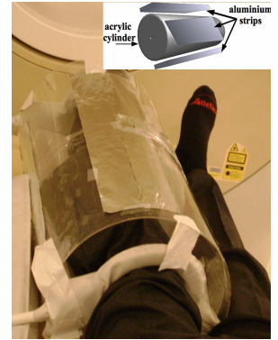
Figure 1. Experimental setup and an illustration of parallel-plate waveguide.
