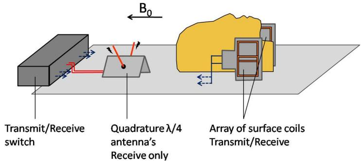
**Fig. 1** Schematic overview of the setup. Two pairs of decoupled RF transceive coils are used for imaging. Two perpendicular  $\lambda/4$  antenna's are used for quadrature reception of a reference acquisition.
