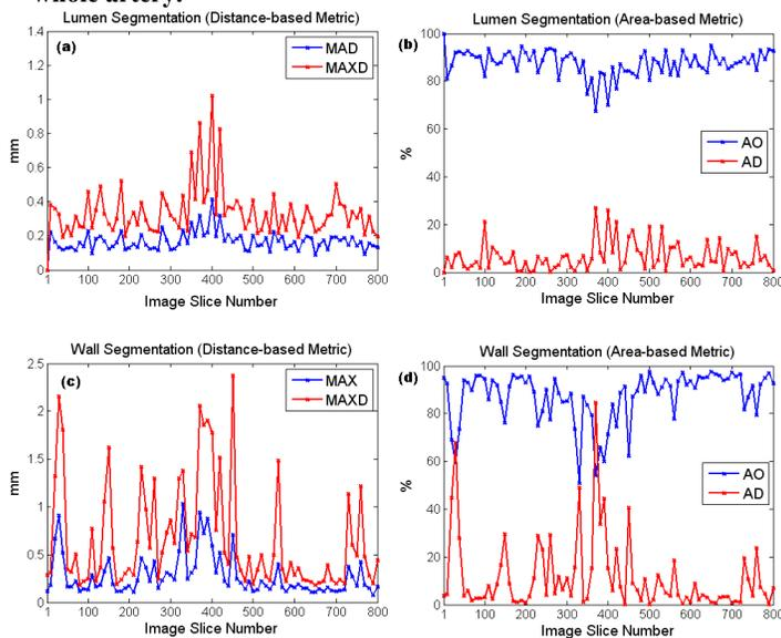
**Fig. 3** MAD, MAXD, AO and AD of the lumen and wall segmentations for 81 images that were manually segmented
