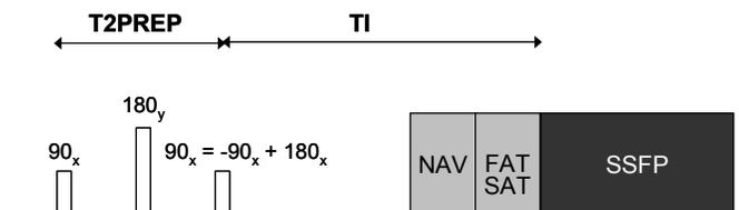
**Fig.1.** 3D T2IR-SSFP sequence for free-breathing BB imaging of the whole chest. Note that all T2IR pulses are spatially non-selective and the  $-90_x$  tip-up of the T2prep sequence and the  $180_x$  inversion pulse can be combined as shown.
