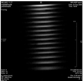
Fig. 6. Image of micro capillary phantom acquired with double microstrip microcoil.
