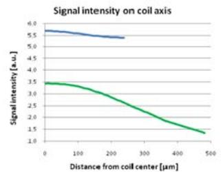
Fig. 3. Distribution of signal intensity along z axis, green line single microstrip, blue line double microstrip
