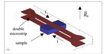
Fig. 2. Double microstrip geometry. Current flows in opposite directions creating uniform  $B_1$  RF field in the volume between strips.
