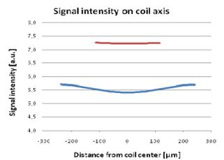
Fig. 4. Distribution of signal intensity along z axis for double microstrip coils having different gap between strips: blue 500  $\mu\text{m}$ , red 250  $\mu\text{m}$ .
