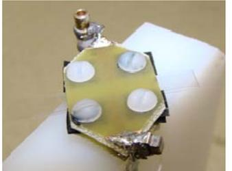
Fig. 5. Double microstrip setup mounted on probehead with sample inserted.
