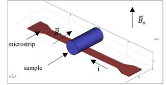
Fig. 1. Single microstrip geometry.  $B_1$  RF field is created by current  $i$  passing through the strip.
