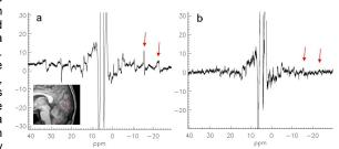
Figure 3: Modulation sidebands in a <sup>1</sup>H spectrum acquired in vivo without water suppression. (a) before, (b) after correction based on field probe data.
