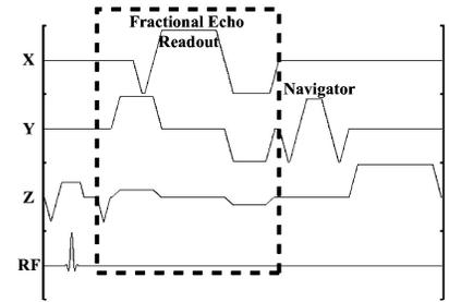
**Figure 1:** Pulse sequence. The dashed frame slides to obtain three different echo times (one per TR) for fat/water separation. The navigator (here on Y) is alternated among the three axes.
