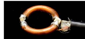
**Figure 2:** 0.5-inch-diameter transmit-receive surface coil used at 7T.
