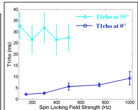
**Fig 3** There is a significant T1ρ dispersion at 0° where T1ρ increased from 2.17 ± 0.07 ms for B1ρ of 100 Hz to 9.33 ± 2.91 ms for B1ρ of 1 kHz, while T1ρ remains largely constant at 55° relative to the B0 field.
