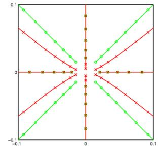
Figure 1: The origin of k-space in the presence of a  $2\mu\text{sec}$  delay on the y gradient relative to the x channel, shown in red compared to the ideal in green. Note the slight curvature of the red trajectory.
