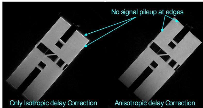
Figure 2. Oblique images reconstructed a) without considering the anisotropy of the physical gradients and b) by mapping the correct physical gradient delays back to the logical (patient) coordinate system. By knowing the three gradient delay parameters, images in all planes can be reconstructed.
