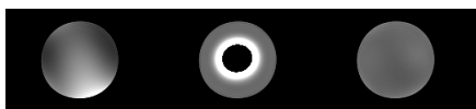
Figure 1. Example of correction of a phantom from left to right (i) image before correction and the corrected images using (ii) ( \lambda = 0 and k=7 ) (iii) ( \lambda = 1e3 and k=7 )
