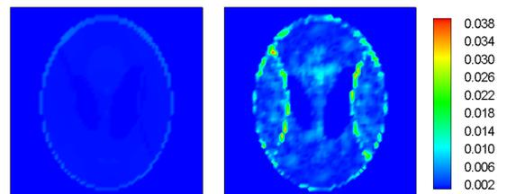
Figure-4 Difference between Original Phantom Image and SENSE-Reconstructed Image by Proposed Method (left) and Polynomial Fit (right)
