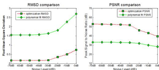
Figure-3 RMSD (left) and PSNR (right) of the Difference between Noise-Free Sensitivity Map and Sensitivity Map Derived by Proposed Method (Red), or Polynomial Fitted (Green)
