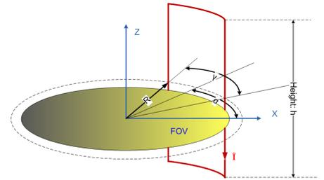
Figure-1 Coil Geometry and Model Descriptors
