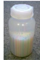
Fig. 1: Phantom with straws in lower part to achieve anisotropic conductivity
