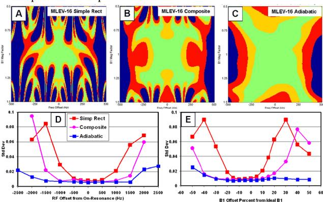
**Fig 1. A-C:** Simulated  $\Delta B_0$  vs.  $\Delta B_1$  longitudinal ( $M_z$ ) T2prep output with green  $\leq 5\%$ , yellow  $\leq 10\%$ , red  $\leq 20\%$ , blue  $> 20\%$  error. **D, E:** Phantom Std Dev (artifacts) under  $\Delta B_0$  and  $\Delta B_1$  conditions.
