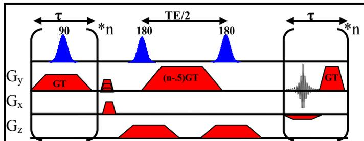
Figure 1: BAR Imaging Sequence. Each excitation pulse excites a particular shape within the field of view according to the pulse profile and the gradient strength. These n subdivisions of the image are then sequentially refocused in the same order they were excited so that each has identical T2 weighting.
