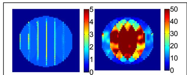
**Figure 3:** G-factor maps for 8 coils, R=8. a) Experimental verification of BAR acquisition with 4 windows effectively creates 32 coils that can be shaped to minimize the G-factor. b) Acquiring the same image in a single window, the G factors are an order of magnitude greater. In both cases, multicoil acquisition is simulated by multiplication with experimental coil profiles.
