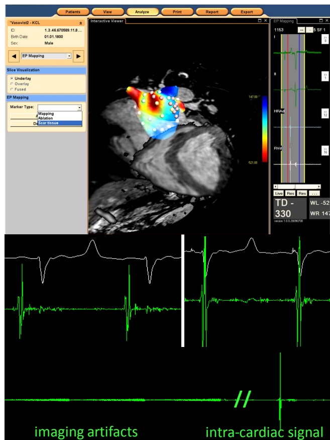
Fig. 1: Top: MR-EP Navigator application. Center: Exemplary in-bore EP recordings at two selected positions showing an atrial signal (left) and a ventricular signal (right). Bottom: Real-time imaging artifacts without filtering in comparison with a typical intra-cardiac signal using HRW [5].
