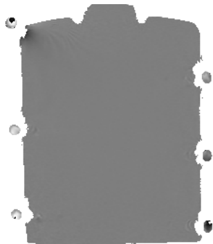
Figure 1, left. Phase change caused by flow. Image: The turns on one side have higher phase than static part of phantom, those on the other side where flow is opposite, lower. Plot: Profile through middle turn at image left showing flow induced phase change in revolutions. As expected, change in static region to the right is only noise.
