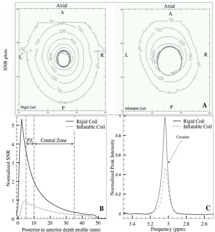
**Figure 1:** (A) A comparison of the rigid coil with the inflatable coil showing SNR as a function of distance in all 3 imaging planes. The bright red regions indicate a more intense signal, while the decaying shades of blue represent decay of the signal. In (B), the normalized SNR versus depth is plotted for both coils. In (C), spectra of creatine obtained from a single voxel experiment demonstrate a ~200% improvement in SNR with the rigid versus the inflatable coil.
