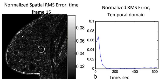
**Figure 2.** (a) Data from digitally simulated enhancing breast was input into I-HYPER algorithm and normalized RMS error image generated (at 158 sec after contrast injection). (b) Normalized RMS error as a function of time.
