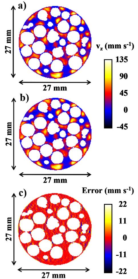
**Figure 1:** a) MR map of the axial velocity of water flowing through a packed bed of 5 mm diameter spheres for full  $\mathbf{k}$ -space sampling. b) Reconstruction of the velocity field in (a) with only 30 % sampling of the full  $\mathbf{k}$ -space distribution. c) Absolute error in the reconstructed velocity distribution.
