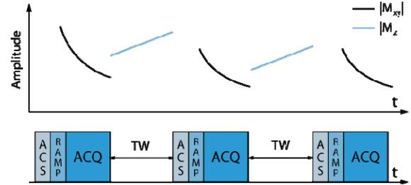
Fig. 1. Imaging scheme used for dynamic MR measurements. TW is defined as a time interval between each image acquisition.
