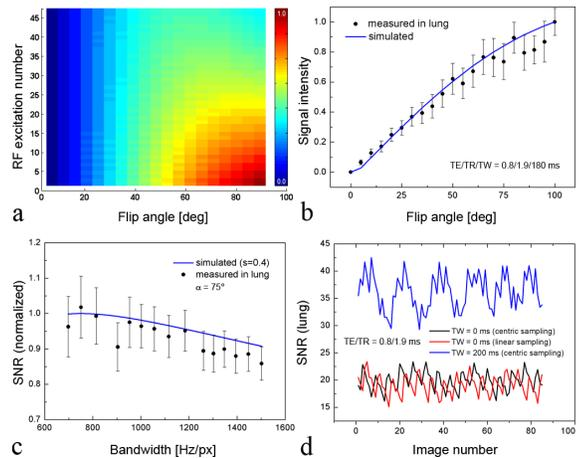
Fig. 2. Diagrams (a) and (b) present simulations and measurements of signal intensity in the lung tissue for different  $\alpha$  values. The SNR as a function of the bandwidth and for various imaging schemes is shown in diagrams (c) and (d).
