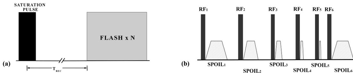
**Figure 1** (a) Timing diagram for saturation-recovery snapshot FLASH (SRSF) and (b) Brix's sequence used as the saturation pulse in (a).
