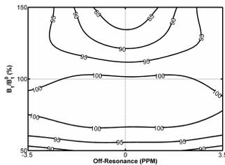
**Figure 2** Simulated relative pulse angle (%) in the presence of RF ( $B_1/B_1^0$ ) and  $B_0$  (off-resonance) inhomogeneities produced using Hoffmann's method of SRSF.
