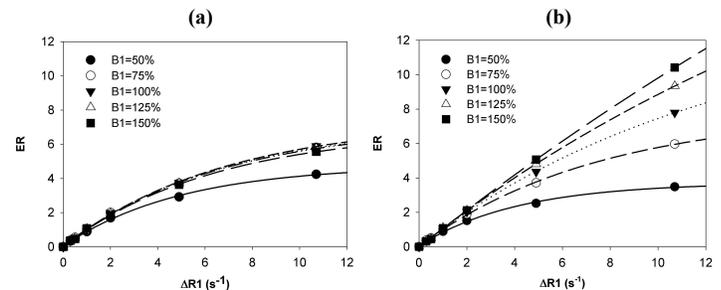
**Figure 3** Enhancement ratio calculated in the presence of RF pulse angle inhomogeneity using (a) Hoffmann's SRSF and (b) standard FLASH.
