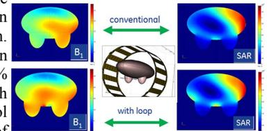
Figure 4: Simulations for  $B_1^{transmit}$  maps (1<sup>st</sup> column) and SAR (2<sup>nd</sup> column) – without (top) and with correction coil (bottom)
