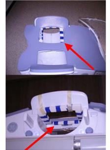
Figure 2: 8 channel breast coil + correction loop (red arrow)
