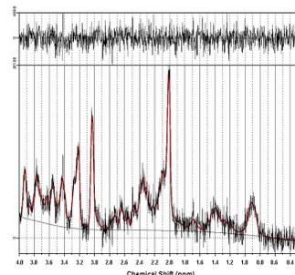
**Fig.3.** Representative *in vivo* proton spectra obtained from left DLPFC of rat using PRESS localization technique. At the top of plot, the residual signal following LCModel fitting is displayed.
