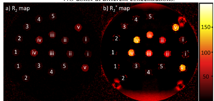
Figure 2. Parameter maps of R_2 (a) and R_2^* (b) obtained from spin- and gradient-echo data respectively. The colour-bar shows relaxation rates in units [ s^{-1} ].
