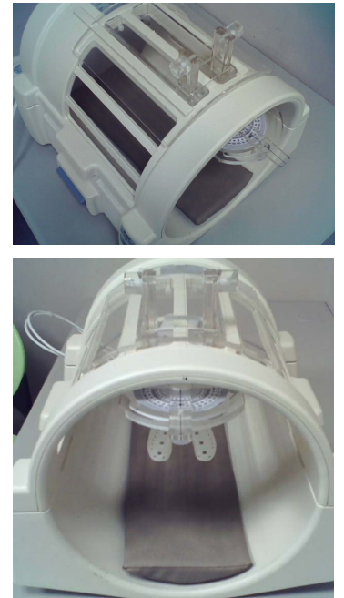
Figure 1. The home-made head holder is allowed rotation along Y axis.. The teeth tray is set at the bottom, and fixed with teeth by dental alginate impression material.
