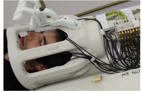
Fig.2: 8-channel head array with integrated 3 rd -order monitoring system. On the right are the four T/R switch- and preamplifier-boards (cf. Fig. 3).
