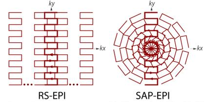
**Fig 1:** K-space trajectories for RS-EPI and SAP-EPI. RS-EPI requires an extra navigator echo for the DW image resulting in reduced scan efficiency, thus SNR, despite that fewer segments are required to fill  $k$ -space. The overlapping blades in the center of  $k$ -space in SAP-EPI may also contribute to a higher  $\eta = SNR / \sqrt{\text{scan time/slice}}$ .
