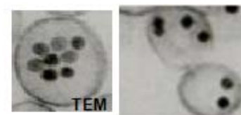
Fig. 3. Electron micrograph of colloidal iron oxide nanoparticles demonstrating the multiple IO crystals incorporated into the oil core of each lipid-encased nanoparticle. Crosslinking (right) appears to discourage aggregation of the particles in the core center as with the non-cross linked version (left).
