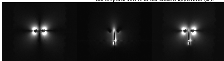
Figure 2: Phantom showing the sensitivity of A) Loop coil B) Loopless coil C) Combined structure
