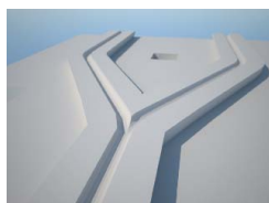
Figure 1: The model bifurcation used in these experiments. The bifurcation was manufactured by AG prototypes using CNC milling techniques. The inner diameter was 0.8mm and the bifurcation angle was 30^\circ .
