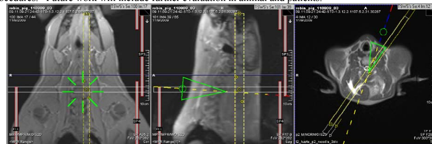
Fig 2. The EndoScout graphic overlay, with real-time tracking updates, is superimposed on the three underlying static slices on the scanner user interface with the tip of the green triangles indicating the needle tip position, and the lines going through the triangles indicating the direction of the needle (yellow: proximal; blue: in-plane and red: distal relative to the respective slices).
