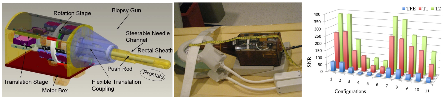
Fig. 1: (a) CAD model of the Transrectal Prostate Intervention, (b) the robot in SNR test setup, and (c) SNR results, averaged for the 10 slices, for the three sequences.
