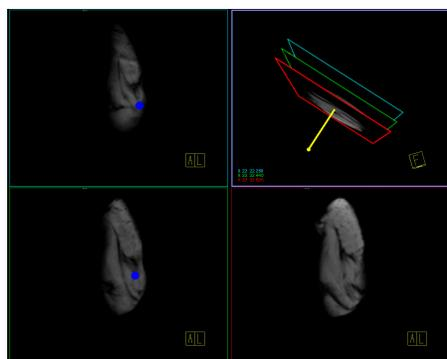
Figure 3: Needle detection module – Real-time, multi-slice imaging perpendicular to the target path is performed during insertion of a needle into a meat sample with successful needle detection (blue circles).
