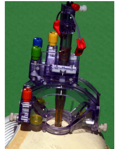
Figure 1: The MR compatible trajectory guide developed for DBS placement and targeted infusion via CED. The guide has an MR visible alignment indicator that has a central lumen through which an electrode or cannula can be inserted. Its orientation can be manipulated around a pivot point and parallel trajectories can be performed with an X-Y translation stage.
