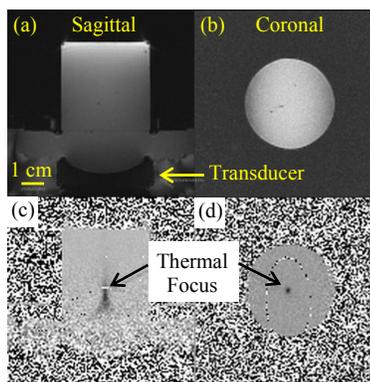
Figure 2: T<sub>1</sub>-weighted images depict the ultrasound transducer positioned directly under the temperature-sensitive phantom in the (a) sagittal and (b) coronal planes. Corresponding MR thermometry images depict the location of the centroid of the thermal focal zone within the phantom in (c) sagittal and (d) coronal planes.
