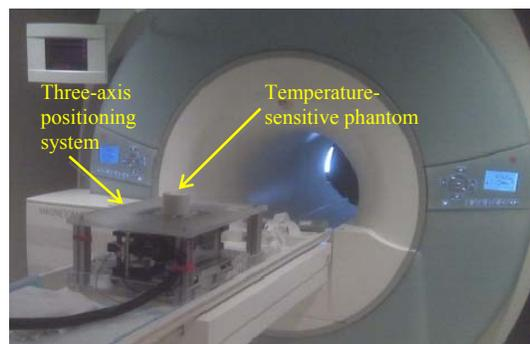
Figure 1: Photograph of the focused ultrasound system installed on a 3.0 T Siemens TIM Trio MR scanner.
