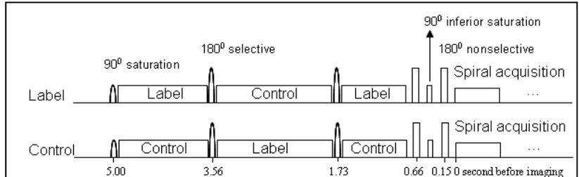
Fig. 2. The interleaved long labeling and background suppression sequence diagram. The selective slab of the  $90^\circ$  saturation pulse and two  $180^\circ$  selective pulses is the imaging volume up to the labeling plane. The  $90^\circ$  inferior saturation pulse is applied to the region below the labeling plane. The control and label block are rapidly repeated gradient and RF pulses for PCASL.
