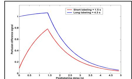
Fig. 1. Theoretical perfusion difference Signals with short labeling period (red) and long labeling period (blue) for the following assumed parameters: transit time 1.4 s, blood  $T_1$  1.65 s, tissue  $T_1$  1.2 s, and perfusion 72 ml/100g.min.
