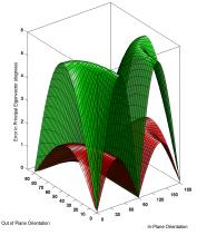
**Figure 1:** Plot of the angular deviation between the true eigenvector orientation and the computed eigenvector orientation when neglecting to account for the volumetric change induced by eddy currents. The horizontal axes correspond to in-plane ( $\theta$ ) and out-of-plane orientation ( $\phi$ ), the vertical axis is the angular deviation. Green and red surfaces correspond to FA = 0.3 and FA = 0.7, respectively. Maxima are of the order of 5° for FA = 0.3, and 1.2° for FA = 0.7
