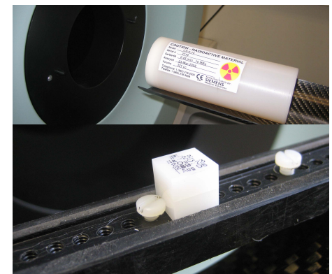
Figure 2. Photographs of diffuse source (top) and point source (bottom) on PET system bed.
