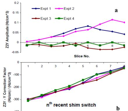
**Fig1 (a): Switching of Z2Y shim, Experiment 1-3 Head phantom; Experiment 4 Spherical phantom (b) Z2Y to Y correction factors.**
