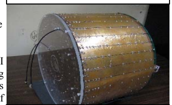
Fig 2: Highpass birdcage RF coil with attached shield and endcap visible.
