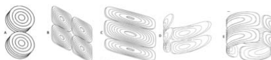
Figure 1: 5 designs. a) Butterfly, b) X-flat, c) Z-flat, d) Half, and e) Cylindrical
