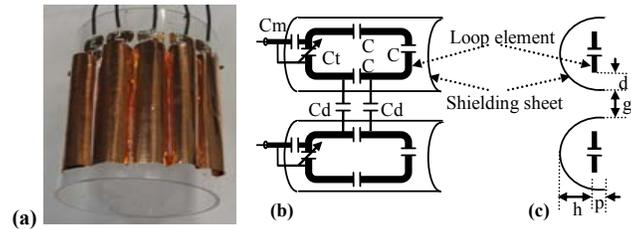
Fig. 1. Decoupling strategy. (a) a photo of the 5-element coil; (b) top view of adjacent elements (c) end view of adjacent elements.
