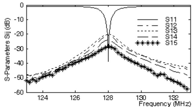
Fig. 3. Measured S-parameters of the constructed 5-element array coil
