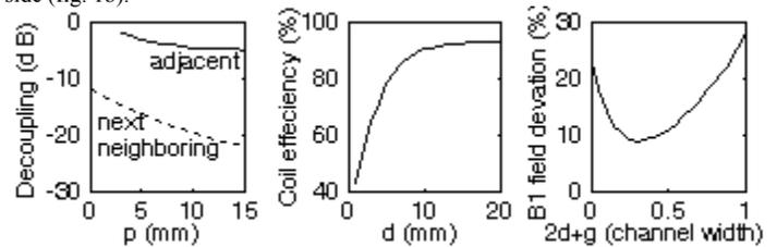
Fig. 2. The effects of parameters of the shielding sheets: (a) decoupling effects vs. penetrating depth; (b) coil efficiency vs. gap; (c)  $B_1$  field deviation vs. gap.
