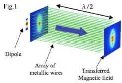
The use of a wire medium in MRI opens several prospects: (i) the possibility to design more reliable endoscopic sensors; (ii) the possibility to create a flexible transmit configuration to excite particular regions with good homogeneity. Hereafter, the properties of wire media are investigated both numerically and experimentally.
