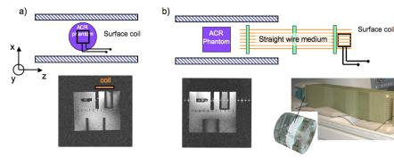
presented in Fig.4.b. A conventional MRI capture of the ACR phantom is presented in Fig.4.a. Both images have approximatively the same signal-to-noise ratio. These results confirm the ability of wire media to transfer MR images with low losses and open the possibility to build new MRI devices devoted to internal imaging.
