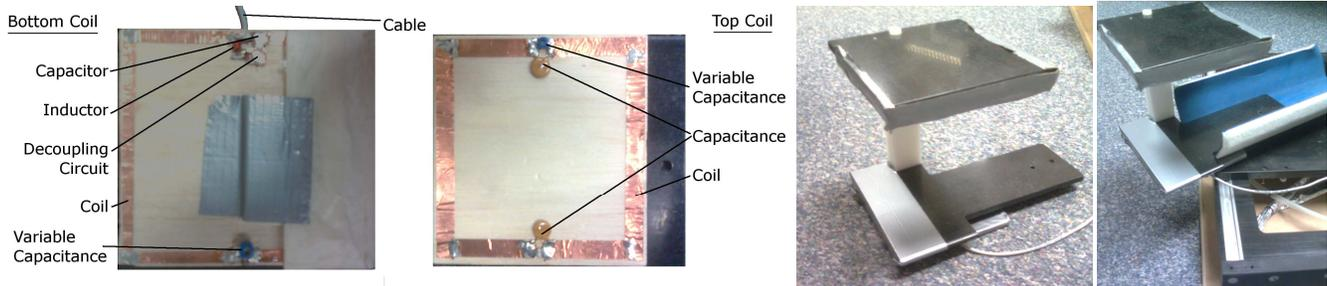
**Figure 1. (Left) The two coil elements. (Right) The coil and the limb-positioning platform. The bottom coil is fixed underneath a plastic base which slides into the gutter attachment of the moveable platform, and is connected to the scanner by a single cable. The top coil is fixed in position by the plastic mount.**
