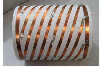
Fig. 1: An 8-leg spiral birdcage coil with total twist of 2\pi .
