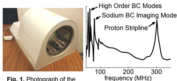
Fig. 1. Photograph of the sodium/proton coil.
