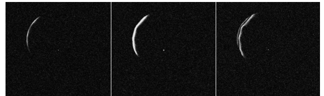
Fig. 3 Curved slice generation using non-selective RF pulses transmitted through an 8-element flexible array wrapped around a 4.1cm diameter phantom. Power was increased from left to right, increasing the depth of excitation. Uniform excitation of a second tipping band is observed at the highest power level.
