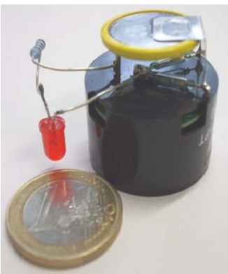
Figure 3: A magneto alert prototype device made from standard electronic components is shown. Of course, even more miniaturized versions are possible, in particular when using a reduced buzzer size. Please note that this prototype included only two reed contacts.
