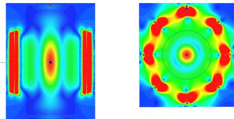
Fig.4.  $B_1+$  profiles. Top: gradient shield included; below: distance to boundary 10mm.
