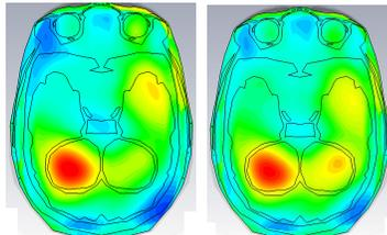
Fig. 2. SAR profile with individual scaling realistic model (left), PEC based (right).
